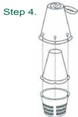
**Step 4.** Place the green outer cone over the black inner cone, making sure that the lid opens in a convenient direction. Line up the screw holes in the base of the green outer cone with the notches on the base of the black inner cone. Use six 10x5/8 self tapping screws to secure the cones to the basket.
