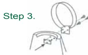
**Step 3.** Place the lid on top of the green outer cone. Screw the hinge to the outer cone using three 10x5/8 self tapping screws and backplate as shown. When using these screws pre-drilled holes are not required.
